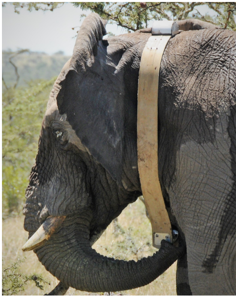
Figure 2: Deployed tracking collar
